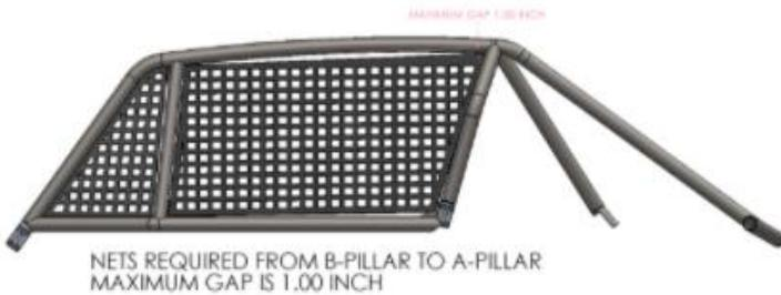
**Window Nets** - Window nets are required from B-Pillar to A-Pillar and that the maximum gap is one (1) inch.
